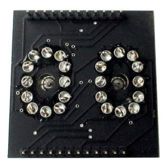
The two straight 12-pin male headers should be inserted into the side of the board opposite the nixie tube sockets. If both of these headers are inserted into the NIXIE DUO board at the same time, they can be the more easily soldered while held in place by the weight of the board.
