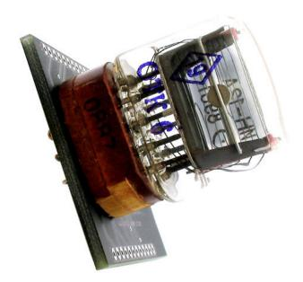
Before inserting nixie tubes or nixie tube sockets, ensure that each nixie tube will be oriented correctly. The numeral 3 is uppermost in the digit stack, and should help make this clear when inserting the nixie tubes into the nixie tube sockets. For nixie tubes that we are currently shipping, pin 1 on each nixie tube is painted white, just inside the tube.
